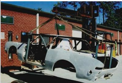
**Avanti Body Lift For Sale** Custom fabrication - specific to Studebaker Avanti only. Bolts together for easy assembly and dismantling. Designed for overhead lifting - allows free working area under the body - an absolute "must" to replace hog troughs properly. Prevents any body flex or deflection while removed, so as to minimize any chance of body cracking. Light weight, yet super-strong.
