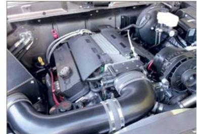
'95 Corvette LT1 small-block backed by a '95 4L60-E four-speed automatic.
